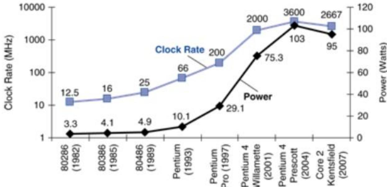
$$\text{Power} = \text{Capacitive load} \times \text{Voltage}^2 \times \text{Frequency}$$
